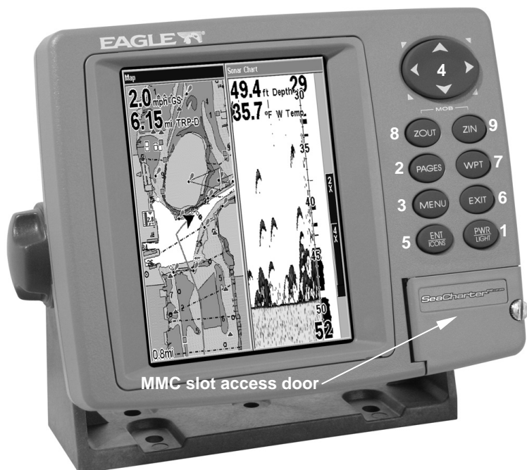
SeaCharter 642cDF iGPS unit showing Map with Sonar page, keyboard and access door for the MMC slot.
